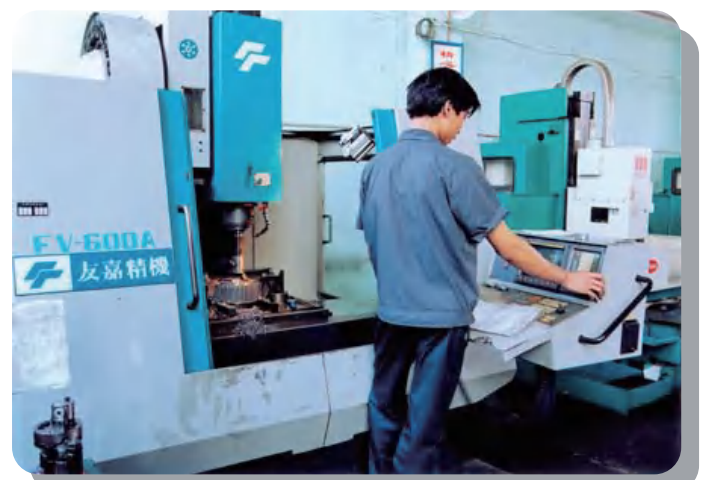
Engineered conveying sprockets made by CNC machining center.
